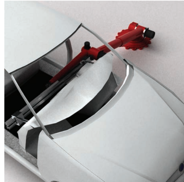
6 The dashboard insertion step, performed by our robot
