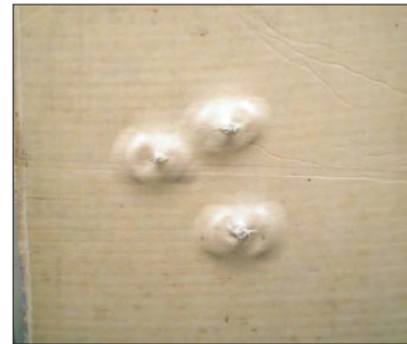
7 Ballistic test on polyethylene composite panel: no penetration with delamination visualisation
