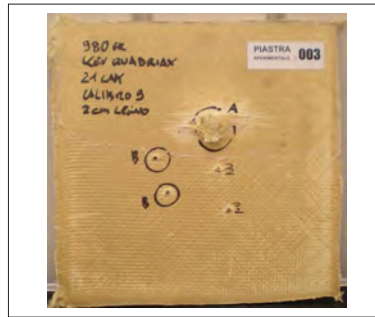
6 Ballistic test on Kevlar® composite panel: full penetration
