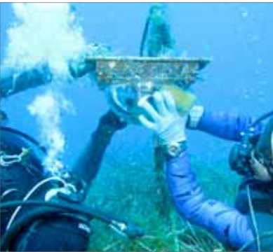
8 Cleaning of the external surface of a dome camera with a common sponge (image by courtesy of Westend s.r.l., http://www.westendpro.com )
