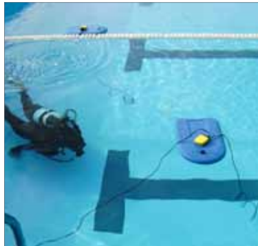
3 Testing the scuba detection algorithm (hydrophones are placed at the bottom)
