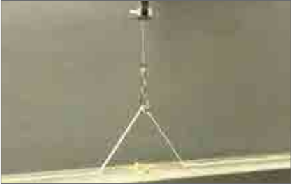
1 Laboratory apparatus to reproduce the condition of detachment of an adhesive tape
