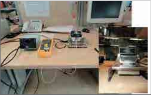
4 Laboratory tests of a Peltier cell for energy harvesting
