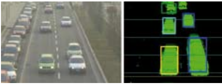
9 The tracking algorithm to count vehicle and determine their speed
