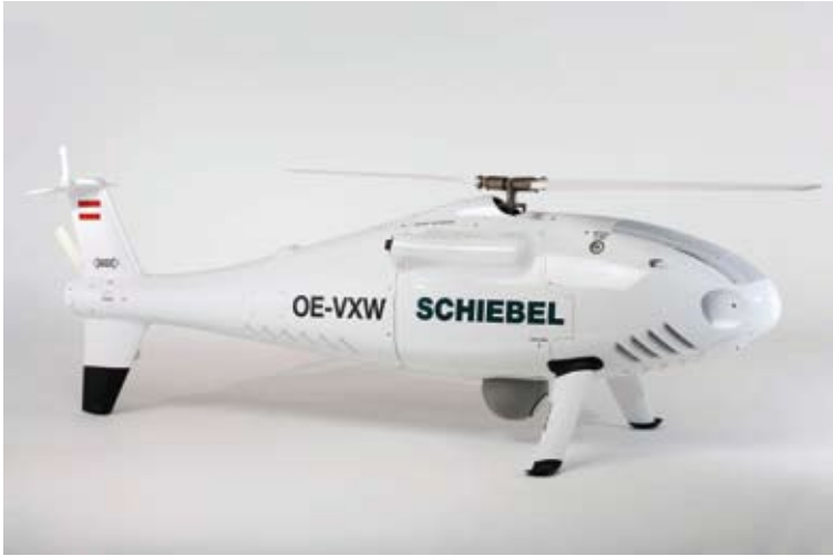
1 The SCHIEBEL CAMCOPTER S-100 is built around a compact helicopter aerial vehicle that can be fitted with a wide variety of payloads tailored to meet diverse user requirements. It is a versatile platform for a great number of applications, both military and civilian
