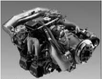
8 Rotax 912 ULS. Engine adopted on the platform developed by AgustaWestland for the CAPECON program
