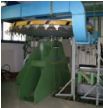
4 Device used for testing ATR95 pantograph
